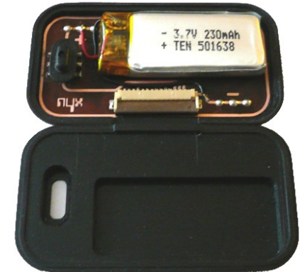
rechargeable battery supply
